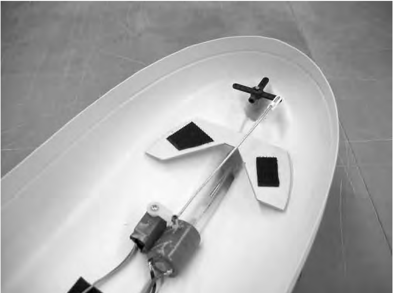
Fig. 2: The interior of the hull with the electric motor installed. The stern tube and coupling sleeve are also in place, as are the rudder and the rudder servo. The shaft support (11) is not shown in this picture.
